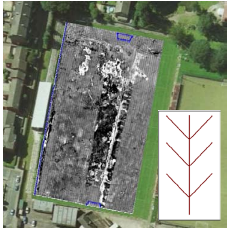
Wakefield football club with GPR data overlay and herringbone drainage system example
